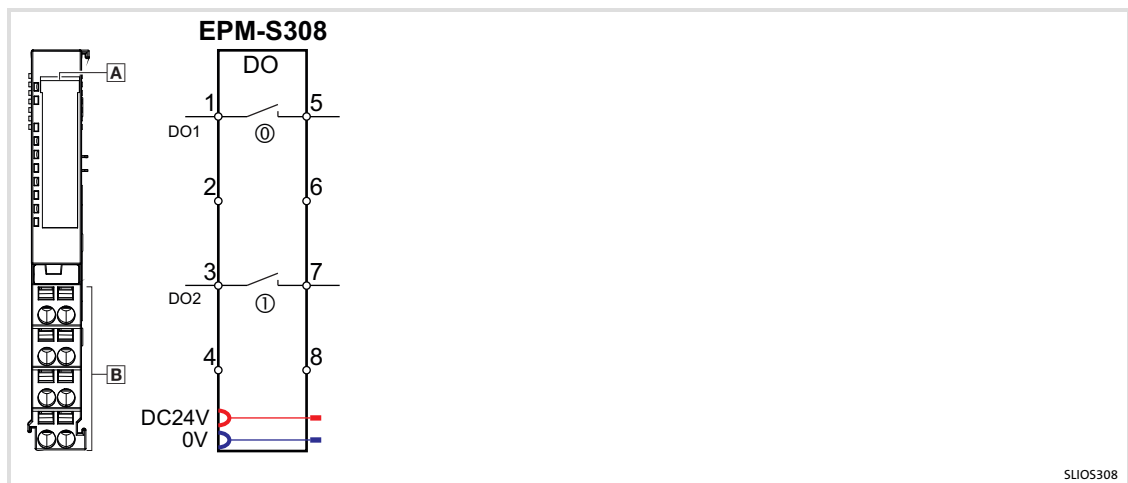
Fig. 3-44 Elements and circuit diagram A Displays for module status B Terminals 1 ... 8 Connection number ① ... ② Bit number in bit presentation
