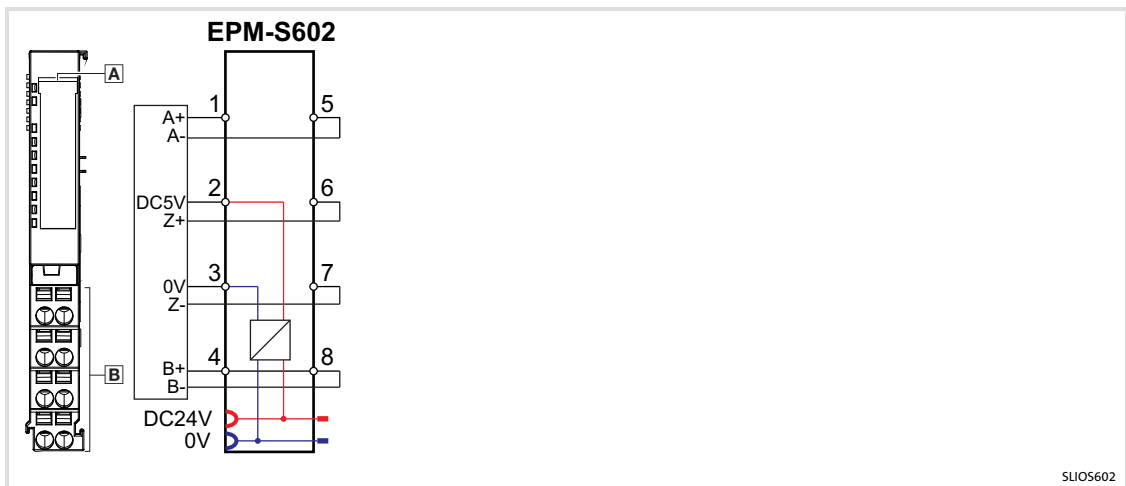
Fig. 3-75 Elements and circuit diagram A Displays for module status B Terminals 1 ... 8 Connection number
