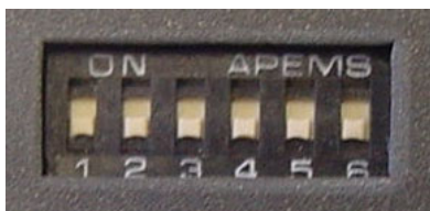
Figure 3-5 Encoder Module DIP Switches
