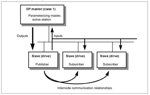
Fig. 6-1 Principle of internode data communication on PROFIBUS-DP
