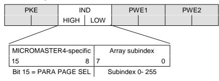
The array subindex is an 8-bit value which is always transferred in the low-order byte (bits 0 to 7) of the parameter index (IND) in acyclical data exchange mode. The Parameter Page Selection task for additional parameters is performed in this case by the high-order byte (bits 8 to 15) of the parameter index. This structure conforms to the USS specification.
