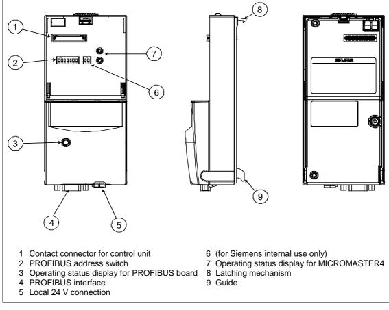
Fig. 1-1 View of communication board
