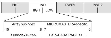
The array subindex (referred to simply as "subindex" in the PROFIDrive Profile) is an 8-bit value which is transferred in the high-order byte (bits 8 to 15) of the parameter index (IND) when data are transferred cyclically via PPOs. The loworder byte (bits 0 to 7) is not defined in PROFIDrive Profile version 2.0. The loworder byte of the parameter index is used on MICROMASTER4 to be able to address additional parameters with a number of >1999.
