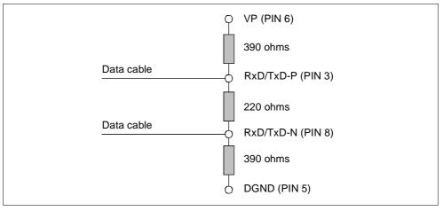
Fig. 4-4 Bus terminating network
