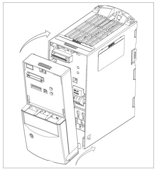
Fig. 4-1 Mounting the communication board on the MICROMASTER4
