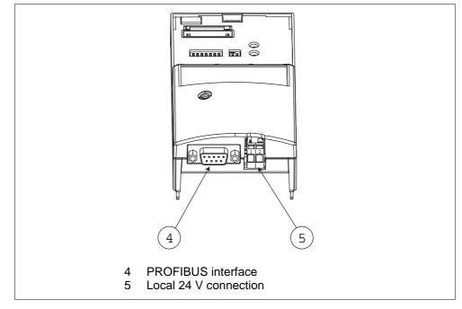
Fig. 4-2 PROFIBUS connection on communication board
