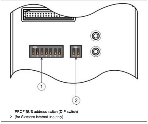
Fig. 5-1 View of DIP switch
