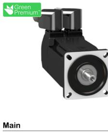
servo motor BMH - 2.5 Nm - 8000 rpm - keyed shaft - without brake - IP54
