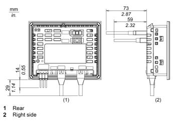
**NOTE:** All the above values are designed with cable bending in mind. The dimensions given here are representative values depending on the type of connection cable in use. Therefore, these values are intended for reference only.
